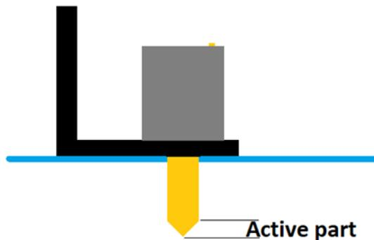
As you can see from the above diagram, lowering water from only the tip and the first 4mm of the bottom of the sensor is all that is needed to trigger the unit.
