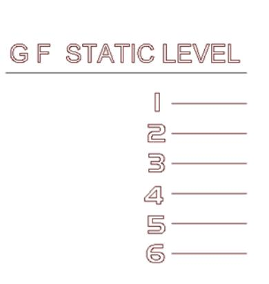
In the above picture, the line under the "G F STATIC LEVEL" is where your pond water level should be, with your circulations pumps switched off. This will maximise the amount of drum you have underwater, increasing available flow rate and time between washes.
