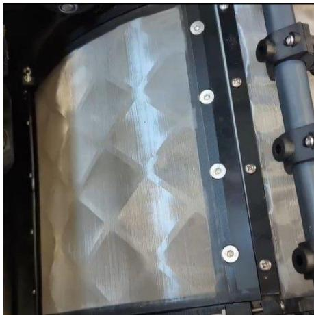
The above pictures show the panel. It can be removed by taking out the 4 bolts on the one edge and once those are undone, then the other end slides out from under the clamp bar. On Gen2 models, there are also 2 bolts on the other end of the panel to remove as well. The panel can then be removed.
