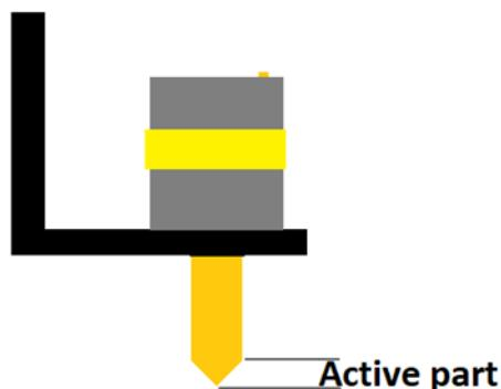
When in operation, in a pump fed system the water level will rise and this will trigger the sensor as the tip is submerged. The integral yellow LED light will come on, showing it is active. The drum will then start its cleaning process, allowing the water level to drop back down, switching the sensor back off and allowing the drum to stop cleaning.
