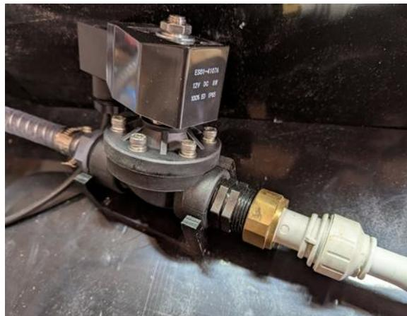
The above example shown with 15mm "speedfit" pipe attached as we do not recommend the use of hozelock hose adaptors. When the water valve closes, it does so immediately, causing a pressure surge in the feed pipe. This surge has been known to "blow off" hozelock fittings, putting the drum into a position where it cannot clean itself.
