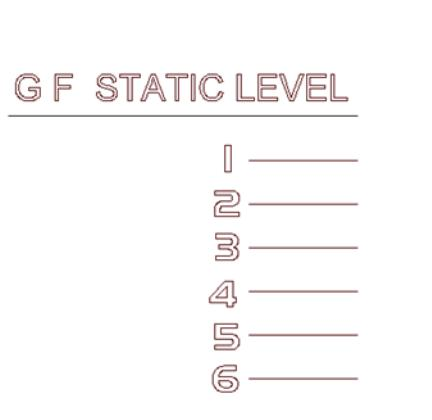
In the above picture, the line under the "G F STATIC LEVEL" is where your pond water level should be, with your circulations pumps switched off. This will maximise the amount of drum you have underwater, increasing available flow rate and time between washes.
