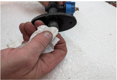
13. Glue the double ended pipe fitting into the end of the spraybar
