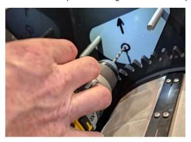
5. Remove the template and the old bolts, then open this hole up to 30mm with a cone drill
