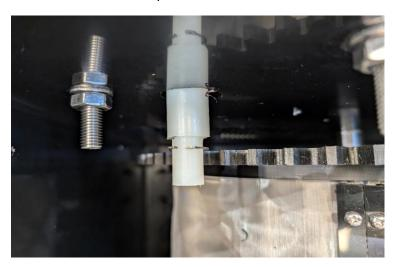
8. Push small drive cog over the shaft, aligning the flat on the shaft with the internal cog hole and secure using the second circlip
