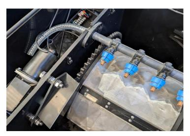
16. Install valve cradle so that the middle of the cradle aligns with the "endplate" of the motor. On Solum units, cradle should be directly under the motor. Drill 2 x 3mm holes through the mounting holes in the cradle and attach with the 2 x 9mm self tappers provided
