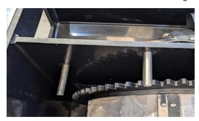
3. Place supplied template over the bolts, with the arrow pointing upward and the markings all facing the drum
