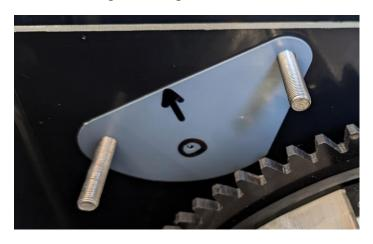
4. Drill a 5mm pilot hole through the hole in the template marked with the ring
