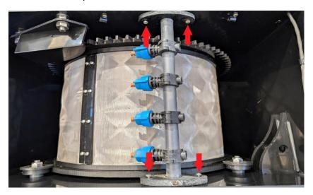
12. Cut off the end of the spraybar, as close to the 90 degree fitting as possible, then clean out the end, making sure to remove any swarf and slimy debris within the end of the tube
