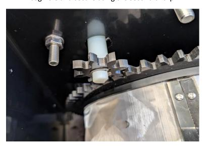
9. Fit finger guard using a washer either side of the guard and secure it with the final 2 M10 nuts provided. It is best attached by putting it over the bottom bolt first and swinging it down to the upper bolt
