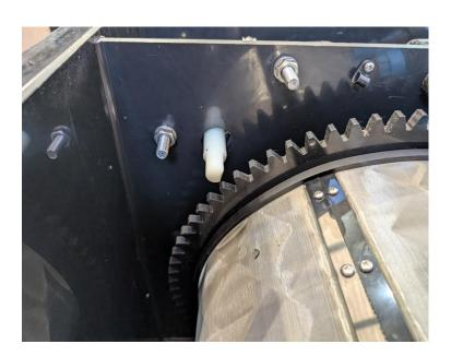
7. Place first circlip inline with the back of the main drum cog
