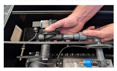
2. Remove the motor wiring from the junction box. Undo and remove the original motor. Undo and remove the rest bolt securing nut, leaving this -
