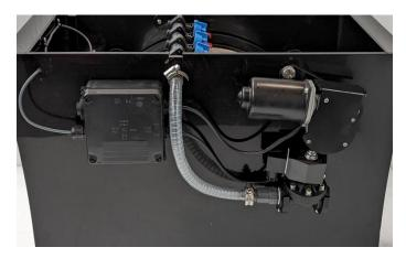
20. Start drum up and press manual wash and check for smooth rotation and also listen to make sure the water valve clicks and no wiring connections have been disturbed.
