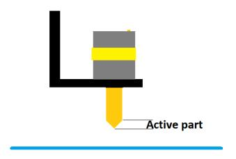
When in operation, in a pump fed system the water level will rise and this will trigger the sensor as the tip is submerged. The integral yellow LED light will come on, showing it is active. The drum will then start its cleaning process, allowing the water level to drop back down, switching the sensor back off and allowing the drum to stop cleaning.
