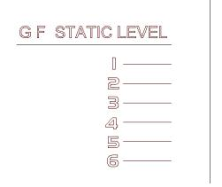
In the above picture, the line under the "G F STATIC LEVEL" is where your pond water level should be, with your circulations pumps switched off. This will maximise the amount of drum you have underwater, increasing available flow rate and time between washes.
