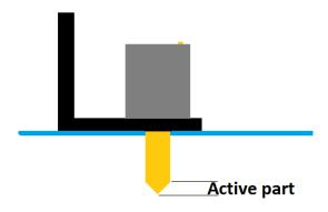
As you can see from the above diagram, submerging only the tip and the first 2 mm of the bottom of the sensor is all that is needed to trigger the unit.
